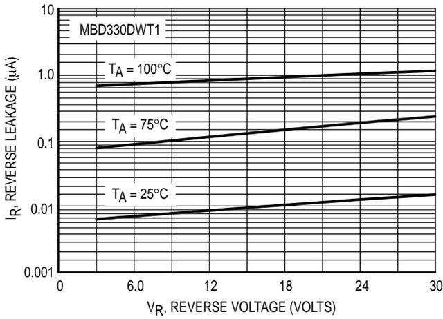
**Figure 8. Reverse Leakage**
