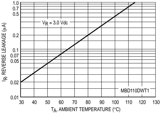
**Figure 1. Reverse Leakage**
