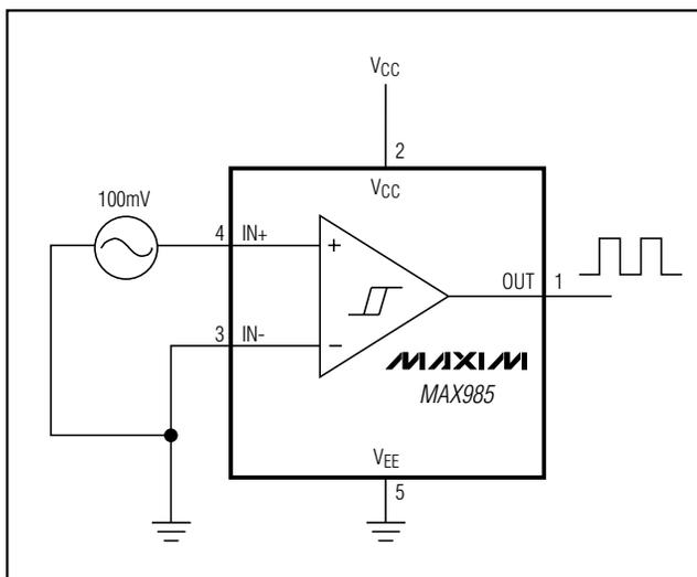
Figure 3. Zero-Crossing Detector
