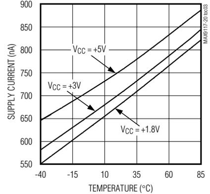
**MAX9119/MAX9120 SUPPLY CURRENT vs. TEMPERATURE**
