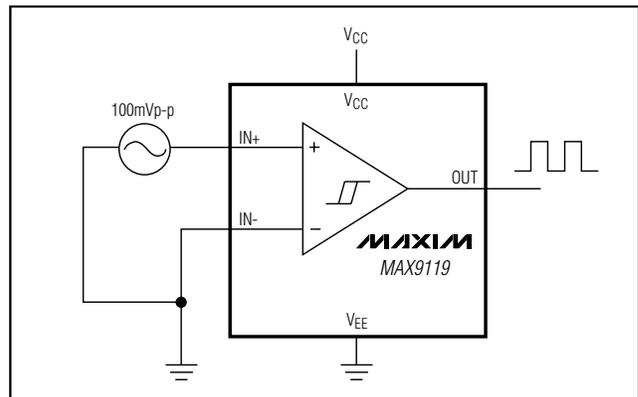
Figure 5. Zero-Crossing Detector
