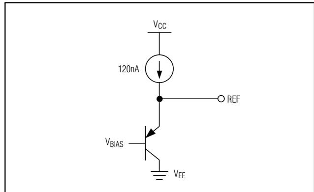
Figure 1. MAX9117/MAX9118 Voltage Reference Output Equivalent Circuit
