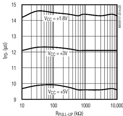
**MAX9118/MAX9120 PROPAGATION DELAY ( $t_{PD+}$ ) vs. PULLUP RESISTANCE**
