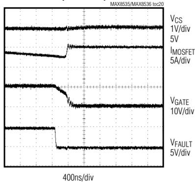
**UVP FAULT WAVEFORM ( $R_1 = 100\Omega$ )**
