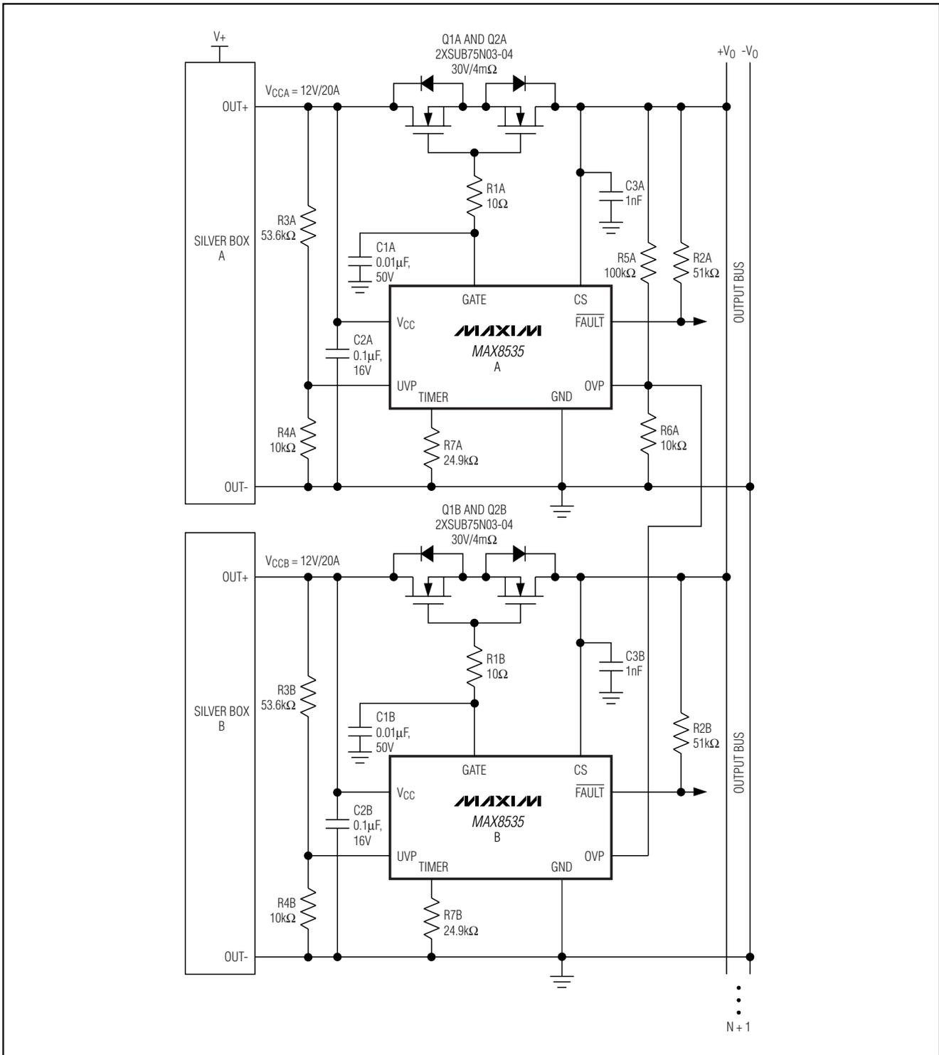
Figure 6. N + 1 Redundant Power System Connections
