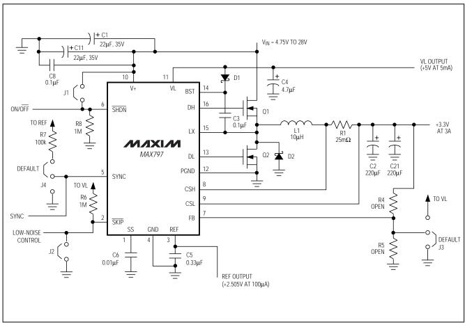
Figure 1. MAX797 EV Kit Schematic
