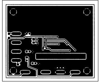
Figure 5. MAX797 EV Kit PC Board Layout—Solder Side
