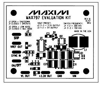
Figure 2. MAX797 EV Kit Component Placement Guide— Component Side
