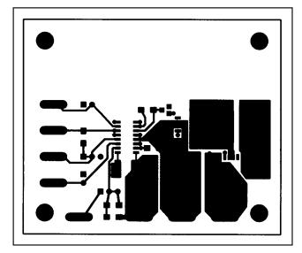
Figure 4. MAX797 EV Kit PC Board Layout—Component Side
