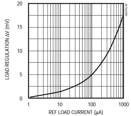
**VL LOAD-REGULATION ERROR vs. LOAD CURRENT**
