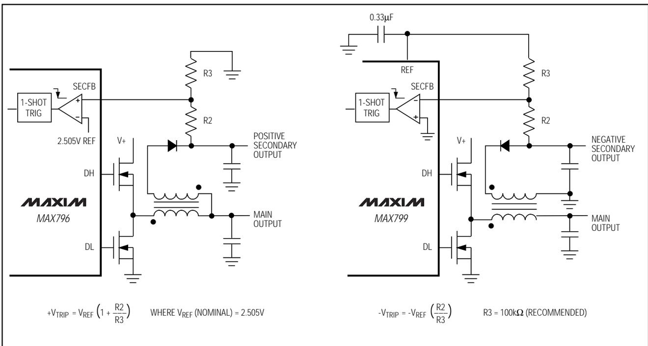
Figure 9. Secondary-Output Feedback Dividers, MAX796 vs. MAX799
