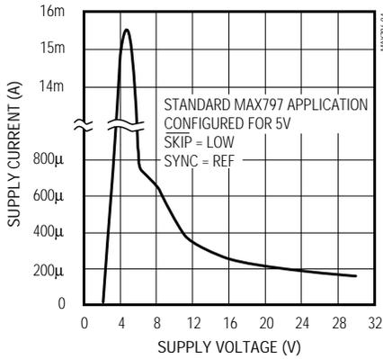
**QUIESCENT SUPPLY CURRENT vs. SUPPLY VOLTAGE, 3.3V/3A CIRCUIT IN IDLE MODE**
