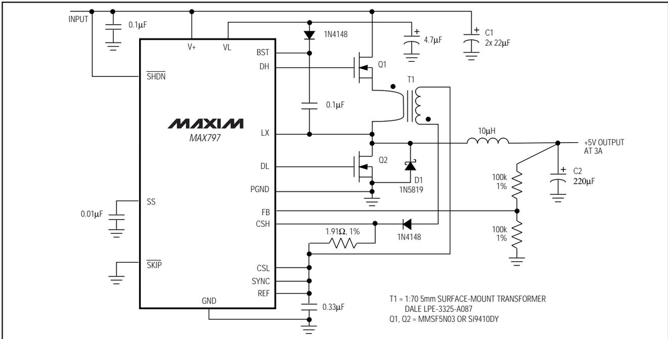
Figure 20. Buck Converter with Low-Loss SMT Current-Sense Transformer
