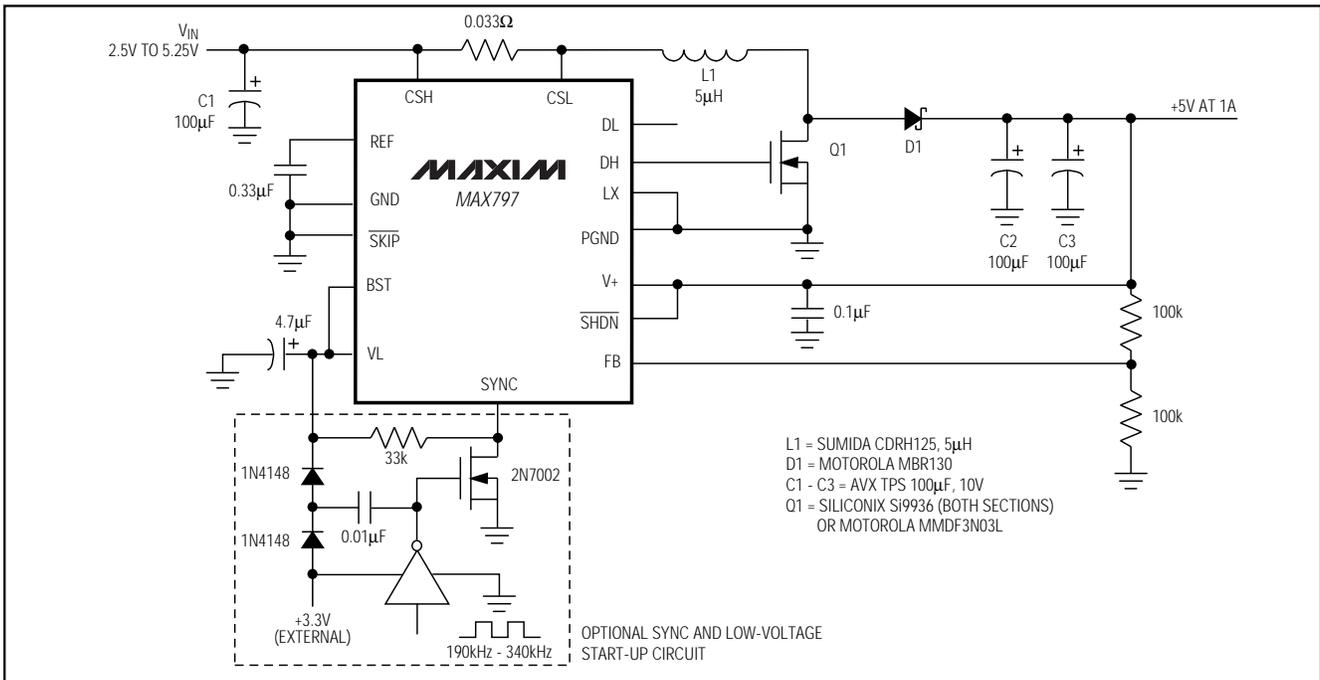
Figure 15. Low-Noise Boost Converter for Cellular Phones
