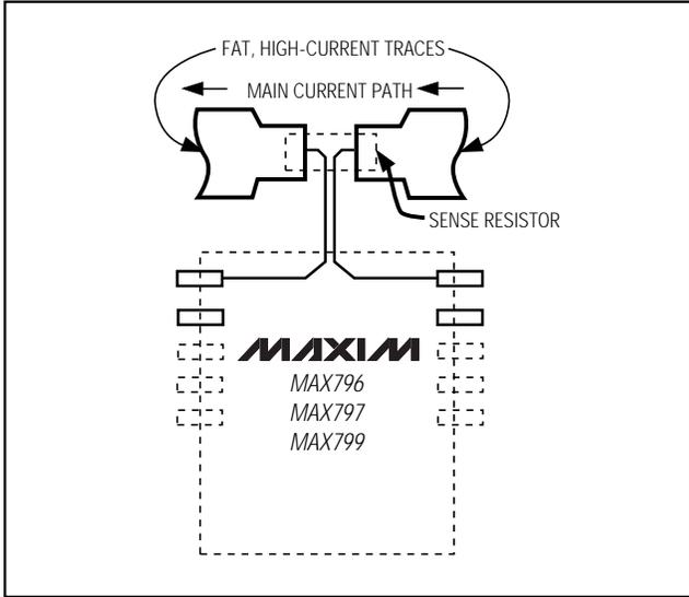
Figure 10. Kelvin Connections for the Current-Sense Resistor
