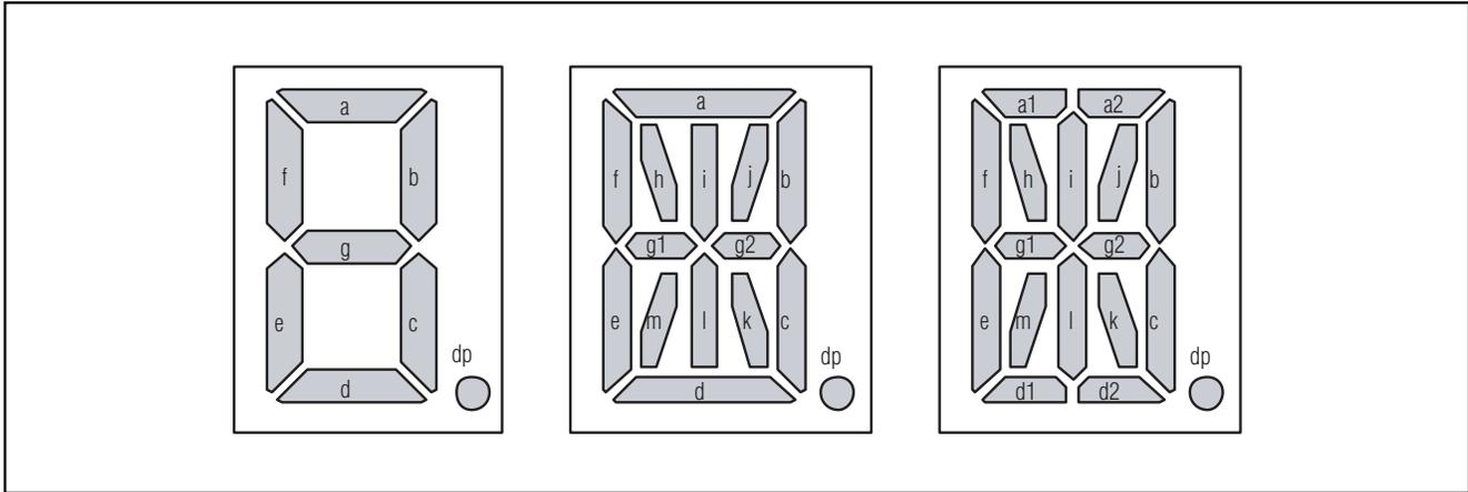
Figure 5. Segment Labeling for 7-, 14-, and 16-Segment Displays
