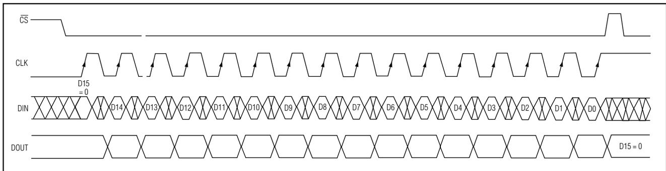
Figure 9. 16-Bit Write Transmission to the MAX6850
