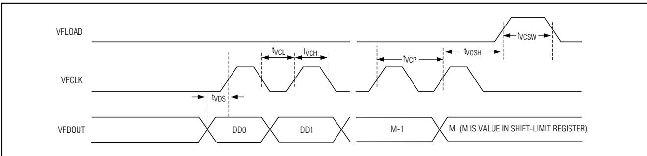
Figure 11. VFD Interface Timing Diagram
