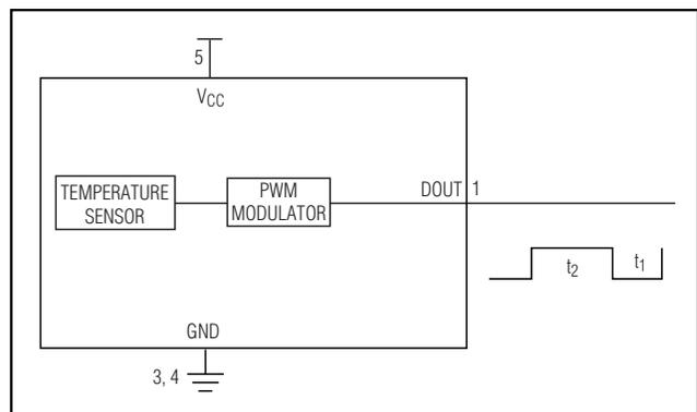
The thermal path between the plastic package and the die is not as good as the path through the leads, so the MAX6672/MAX6673, like all temperature sensors in plastic packages, are less sensitive to the temperature of the surrounding air than they are to the temperature of their leads. They can be successfully used to sense ambient temperature if the circuit board is designed to track the ambient temperature.
