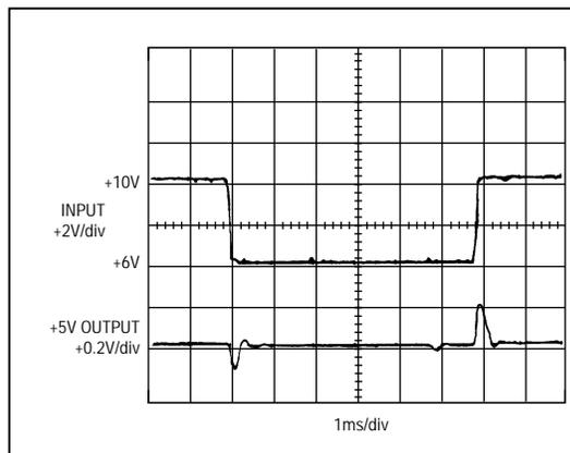
Figure 11. Output Response to +4V/100µs Input Step
