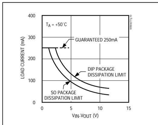
Figure 10. MAX667 Load Current vs. Input-Output Differential Voltage
