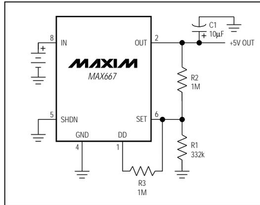
Figure 7. Connection for Minimum Quiescent Current Near Dropout
