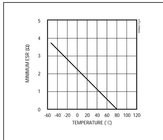
Figure 4. Minimum Required Output-Capacitor ESR vs. Temperature
