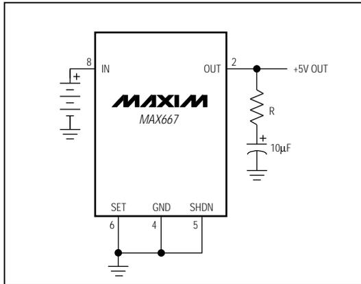
Figure 5. Alternative Stability Scheme Using Resistor R
