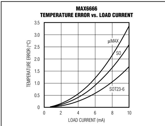
Figure 3. MAX6666 Temperature Error Due to Load Current
