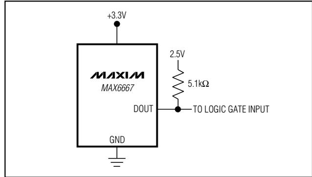
Figure 4. Low-Voltage Logic
