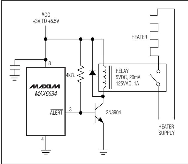
Figure 10. Simple Thermostat
