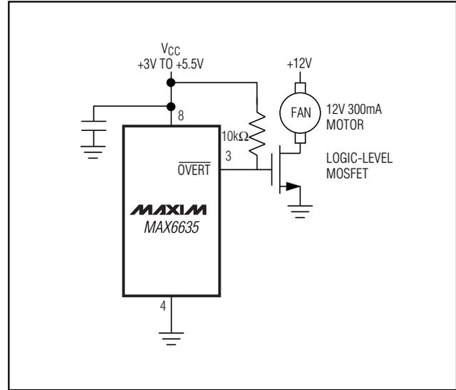
Figure 11. Fan Controller
