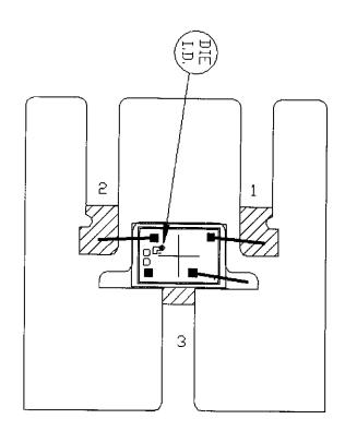
NOTE: USE NON-CONDUCTING EPOXY DIE ATTACH
