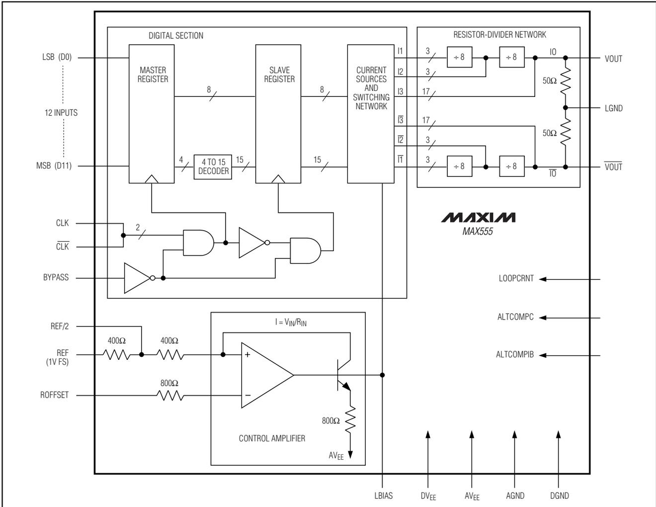
Figure 1. Functional Diagram
