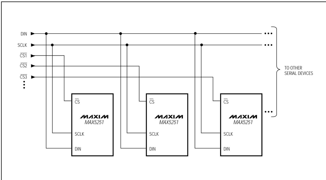
Figure 8. Multiple MAX5251s Sharing a Common DIN Line
