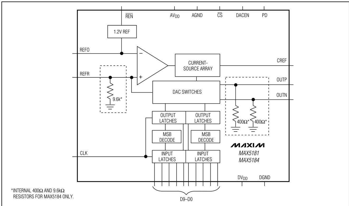
Figure 1. Functional Diagram
