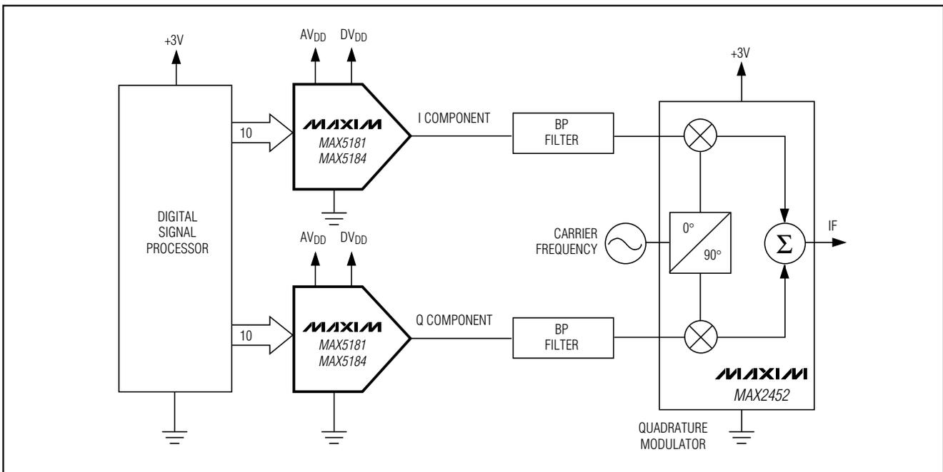
Figure 7. Using the MAX5181/MAX5184 for I/Q Signal Reconstruction
