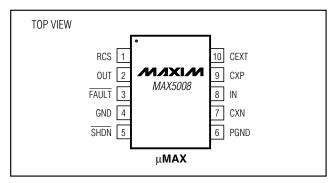
low-impedance trace, and connect the ground for  $C_{\mbox{\footnotesize{IN}}},$   $C_{\mbox{\footnotesize{EXT}}},$  and  $C_{\mbox{\footnotesize{OUT}}}$  directly to PGND in a star configuration. Connect RCs to  $C_{\mbox{\footnotesize{EXT}}}$  through a short and low impedance trace.
