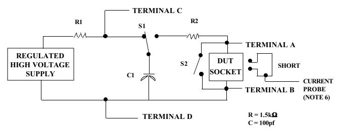
and output pins connected to terminal B. All pins except the input or output pin being tested and the combination of all the Mil Std 883D other input and output pins shall be open.
