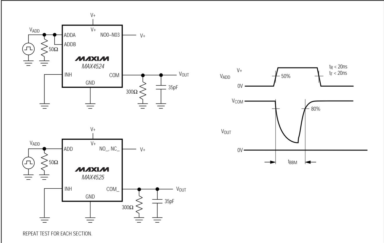
Figure 3. Break-Before-Make Interval
