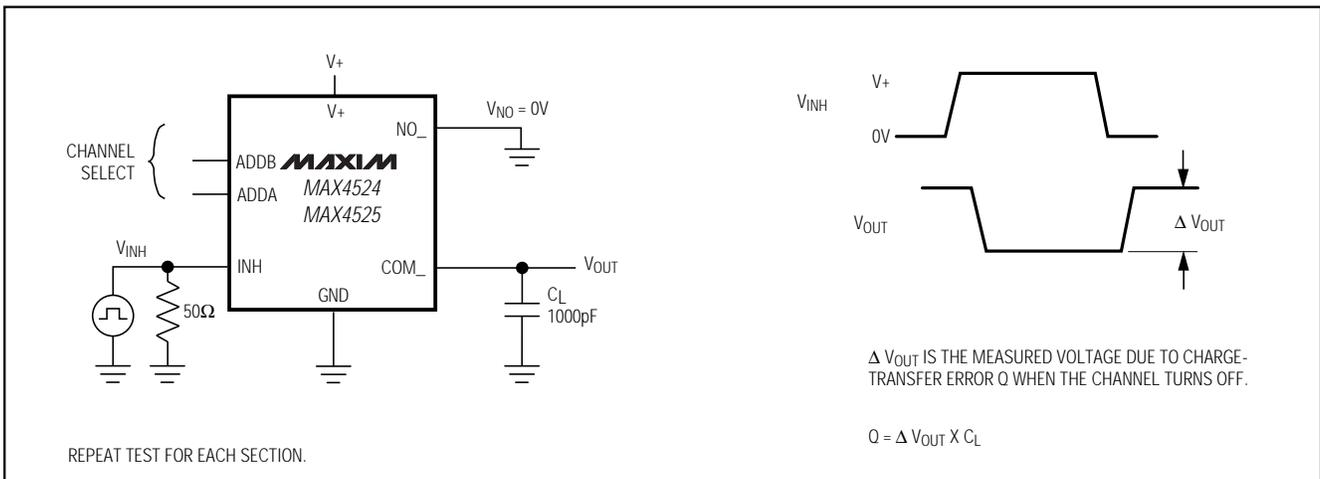
Figure 4. Charge Injection
