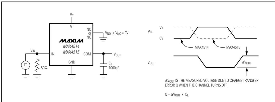
Figure 1. Charge Injection
