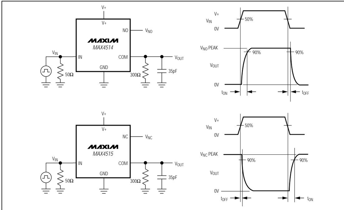
Figure 2. Switching Times
