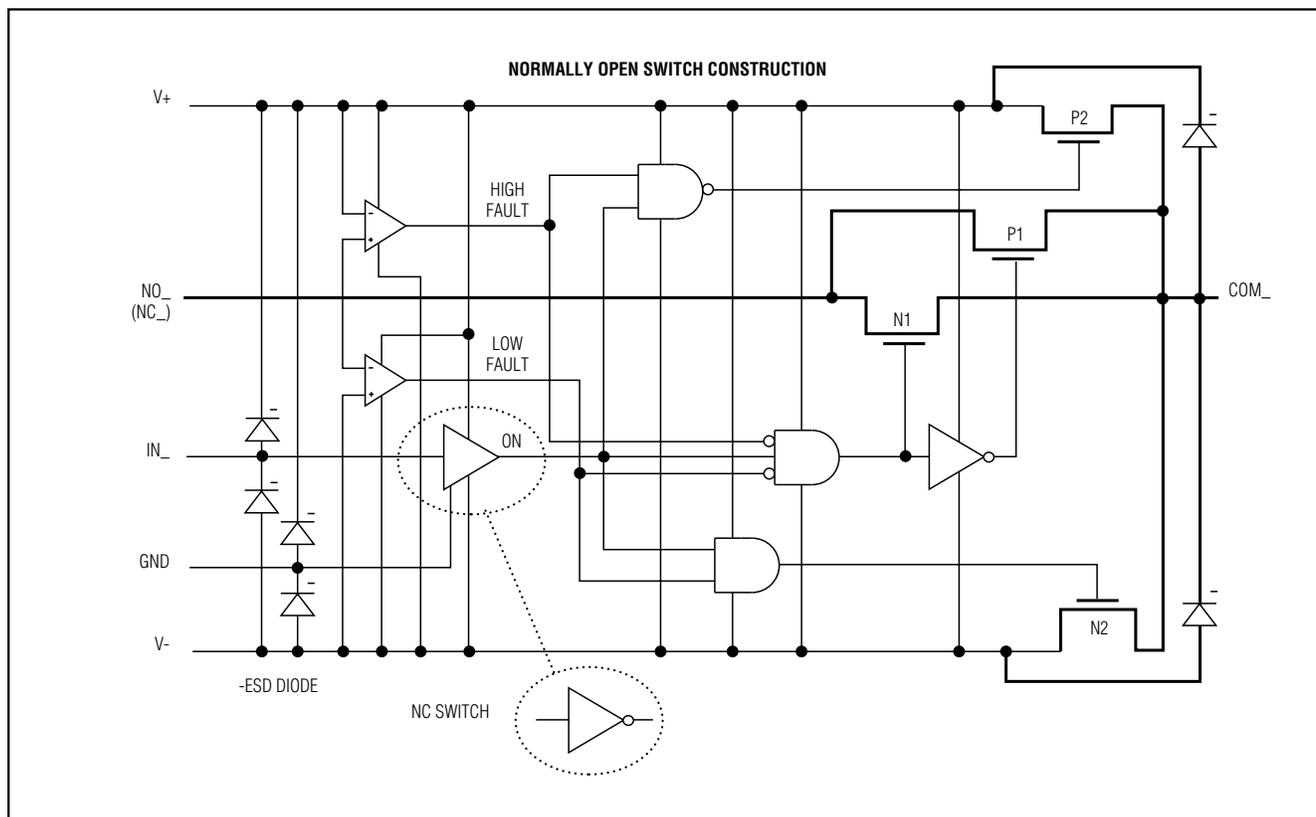
Figure 1. Block Diagram
