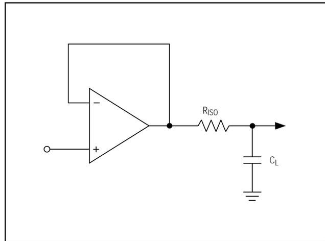
Figure 11. Capacitive-Load-Driving Circuit
