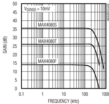
**MAX4081F/T/S SMALL-SIGNAL GAIN vs. FREQUENCY**
