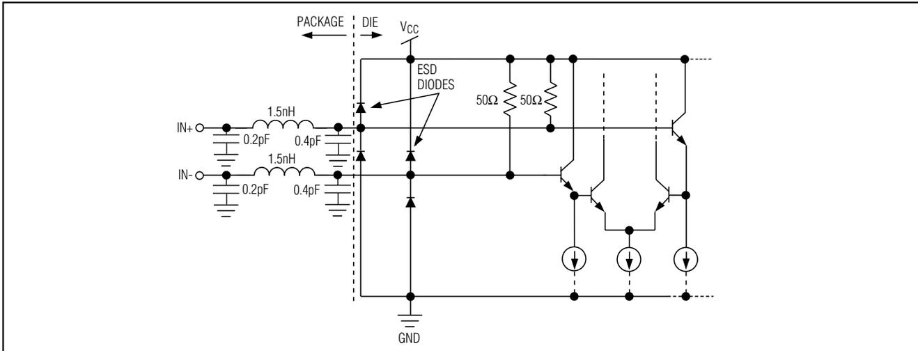
Figure 2. Input Structure
