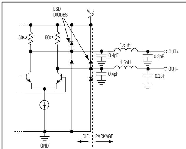
Figure 3. Output Structure
