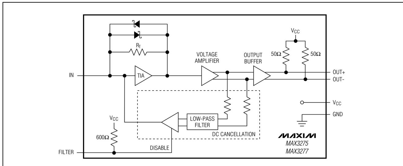
Figure 1. Functional Diagram
