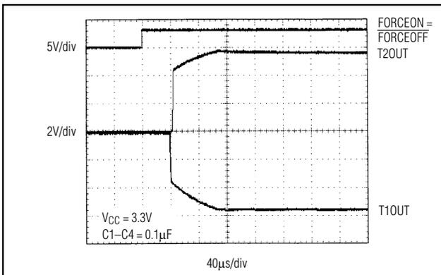
Figure 8. Transmitter Outputs Exiting Shutdown or Powering Up
