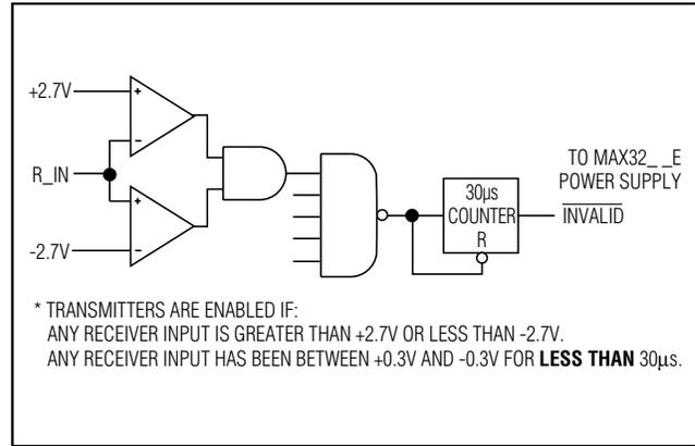
Figure 3b. MAX32\_E with Transmitters Enabled Using AutoShutdown
