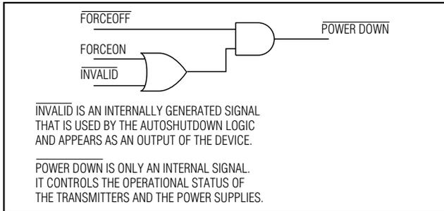
Figure 3c. MAX3221E AutoShutdown Logic
