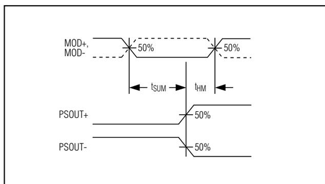
Figure 1. Timing Diagram
