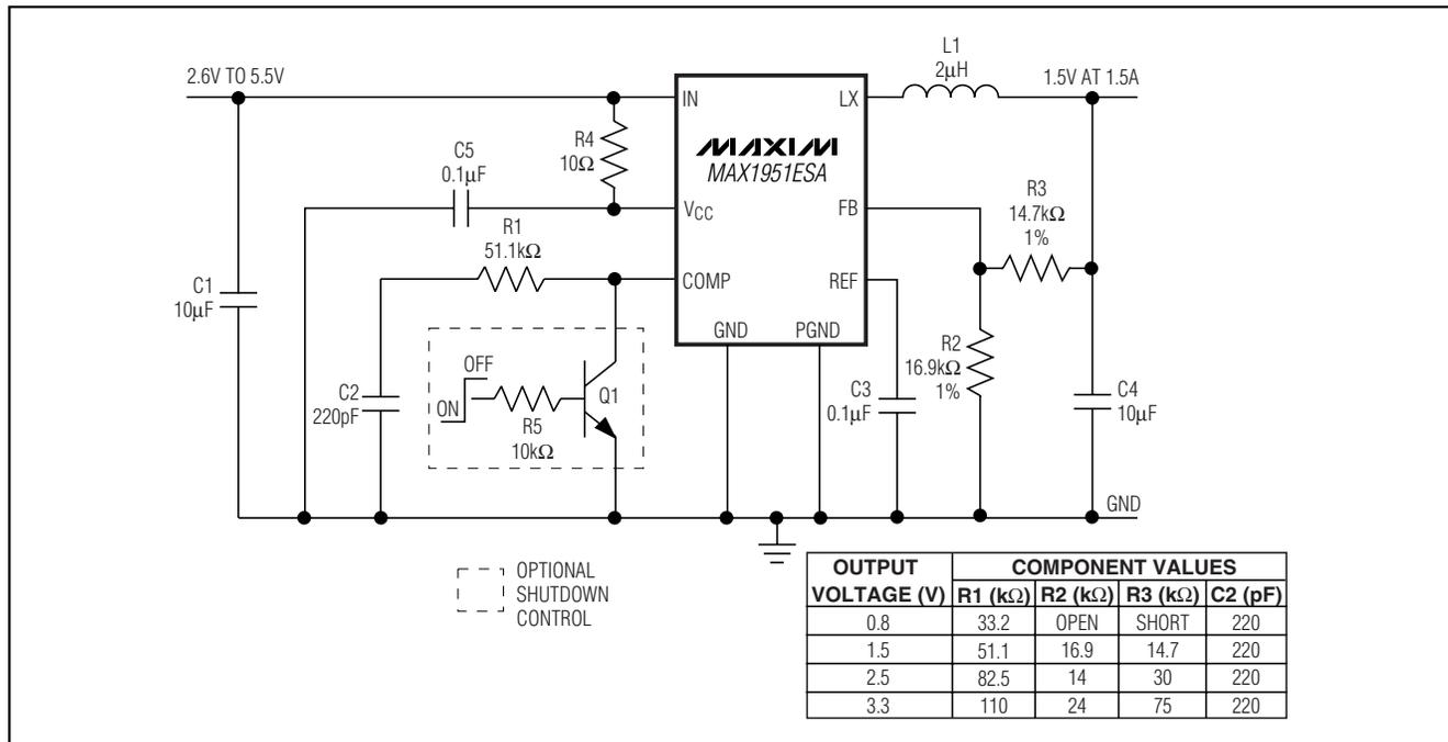
Figure 2a. MAX1951 Adjustable Output Typical Application Circuit
