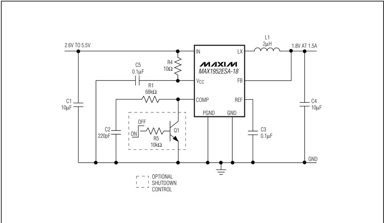
Figure 2b. MAX1952 Fixed-Output Typical Application Circuit
