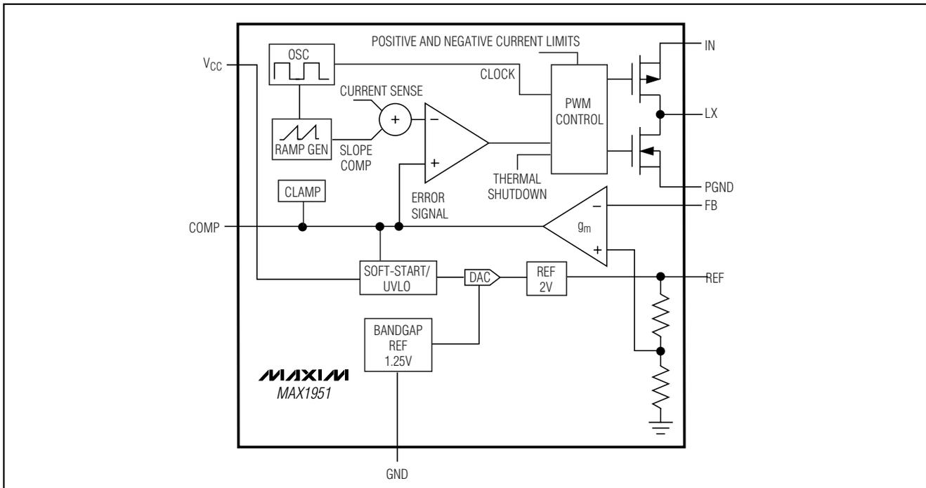
Figure 1. Functional Diagram
