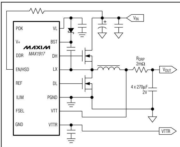
Figure 1. Using a Resistor for Voltage Positioning
