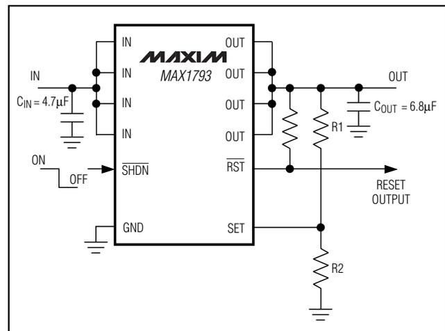
Figure 3. Typical Operating Circuit with Adjustable Output Voltage
