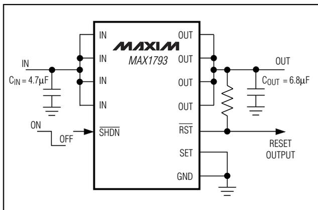
Figure 2. Typical Operating Circuit with Preset Output Voltage
