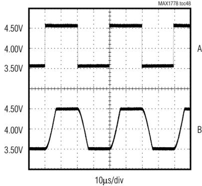
A.  $V_{BUF+} = 3.50V$  TO  $4.50V$ ,  $0.5V/div$
