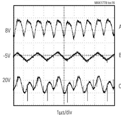
A.  $V_{MAIN} = 8V$ ,  $I_{MAIN} = 200mA$ , 10mV/div
