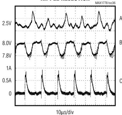
A.  $V_{LDO} = 2.5V$ ,  $I_{LDO} = 200mA$ , 10mV/div
