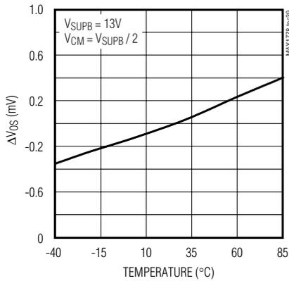
**INPUT OFFSET VOLTAGE DEVIATION vs. TEMPERATURE**
