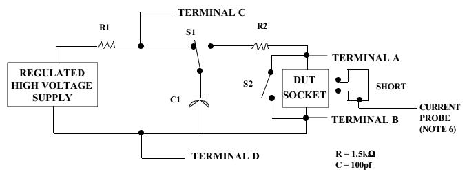
Mil Std 883D Method 3015.7 Notice 8 c. Each input and each output individually connected to terminal A with respect to a combination of all the other input and output pins connected to terminal B. All pins except the input or output pin being tested and the combination of all the other input and output pins shall be open.
