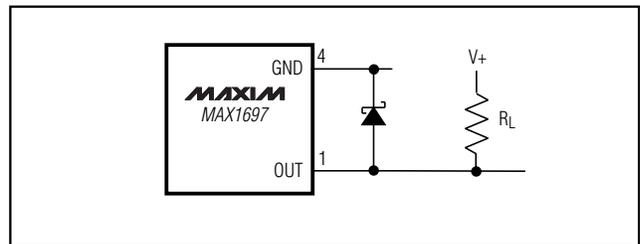
Figure 7. Heavy Load Connected to a Positive Supply
