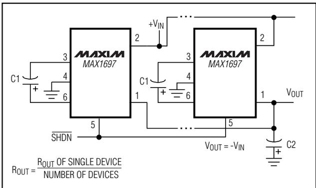
Figure 5. Paralleling MAX1697s to Reduce Output Resistance
