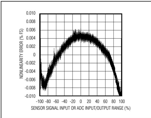
Figure 2a. Analog Front-End Integrated Nonlinearity (INL) (typ)
