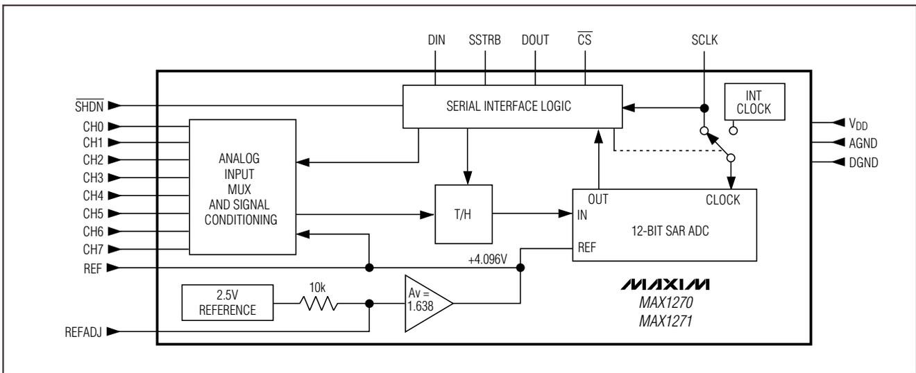
Figure 3. Block Diagram
