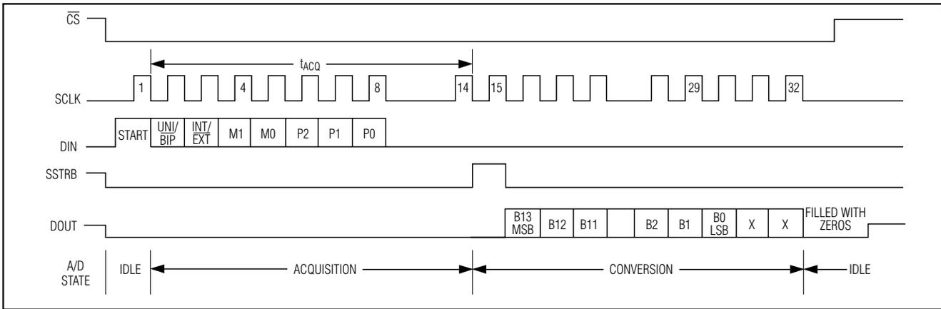
Figure 3. Long Acquisition Mode (32 Clock Cycles) External Clock
