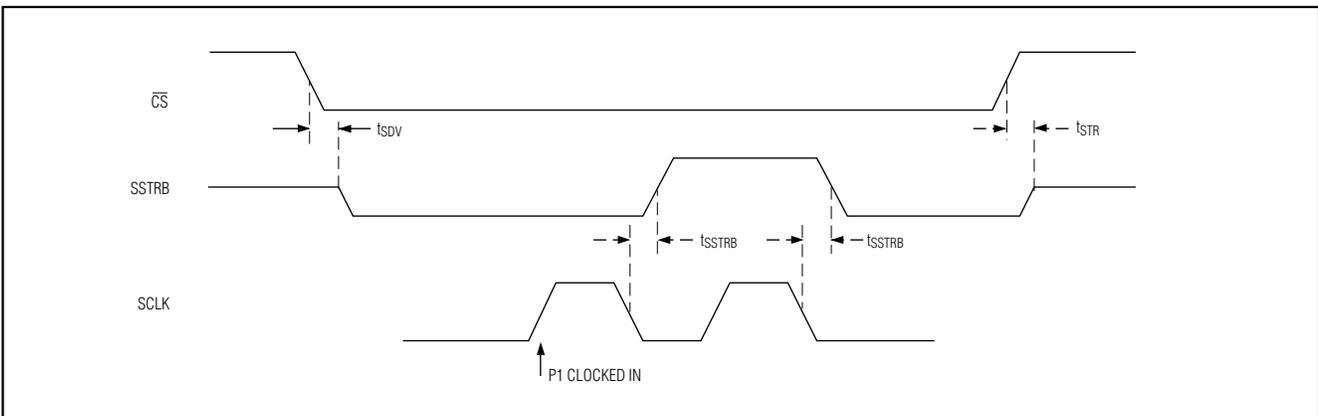
Figure 4. External Clock Mode SSTRB Detailed Timing
