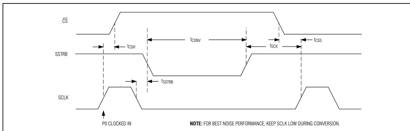
Figure 6. Internal Clock Mode SSTRB Detailed Timing
