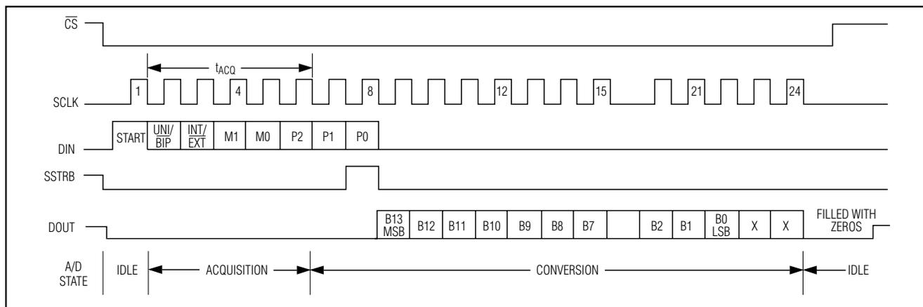
Figure 2. Short Acquisition Mode (24 Clock Cycles) External Clock
