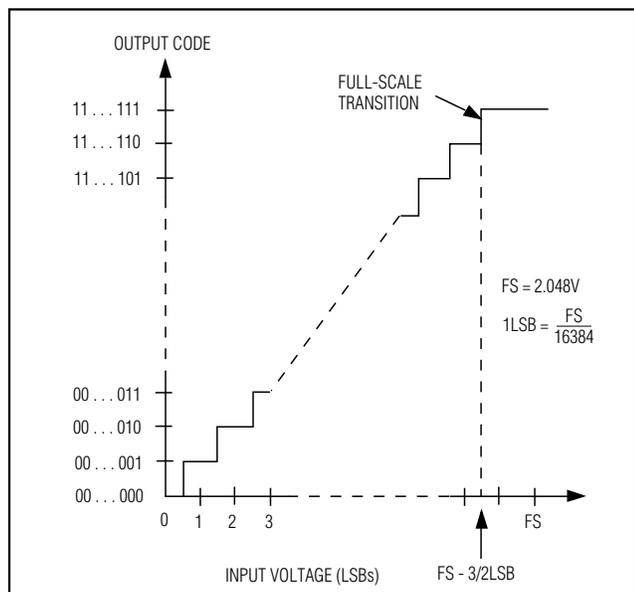
Figure 8. MAX1145 Unipolar Transfer Function, 2.048V = Full Scale
