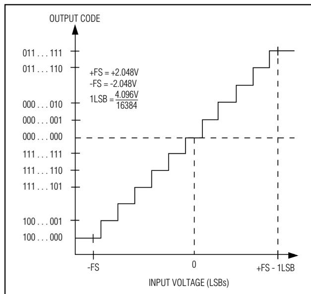
Figure 9. MAX1145 Bipolar Transfer Function, 4.096V = Full Scale
