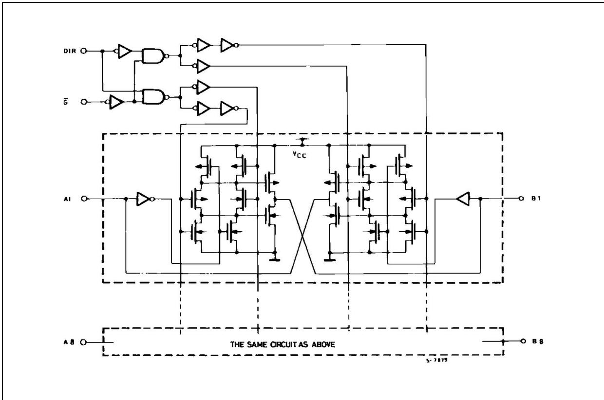
This logic diagram has not be used to estimate propagation delays
