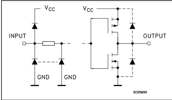
**INPUT AND OUTPUT EQUIVALENT CIRCUIT
