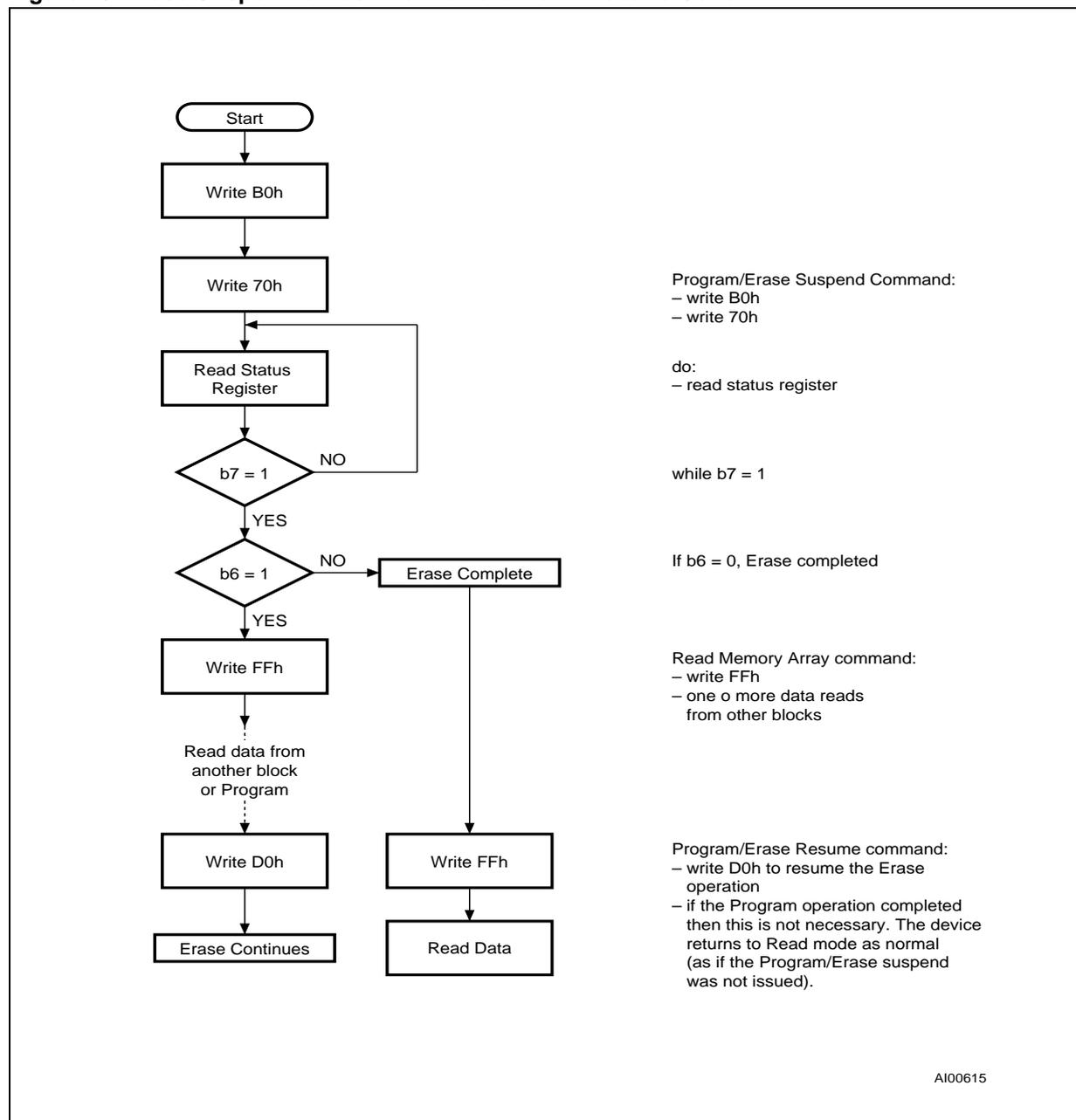
Figure 30. Command Interface and Program Erase Controller Flowchart (b)
