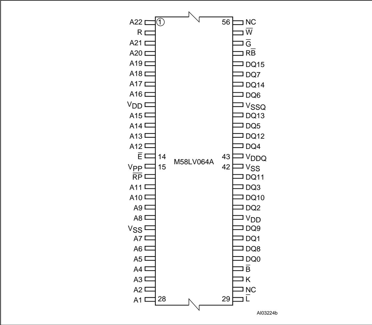
Figure 4. TBGA64 Connections for M58LV064A (Top view through package)
