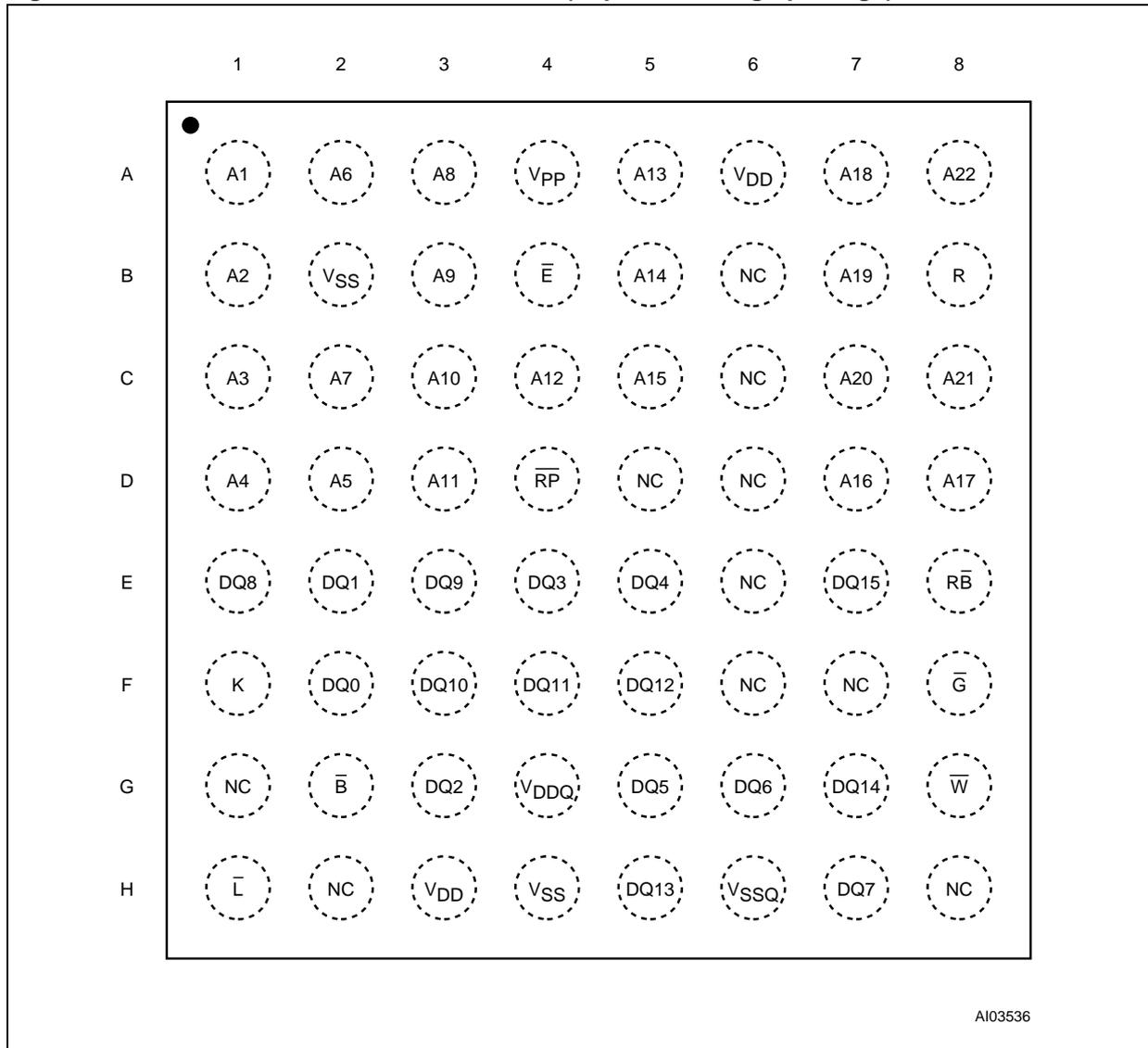
Figure 5. TBGA80 Connections for M58LV064B (Top view through package)
