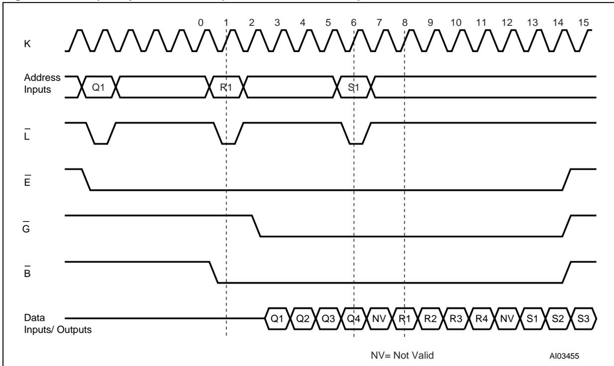
Note: In this example the Burst Configuration Register is set with M2-M0 = 001 (Burst Length = 4 Words or Double Words), M6 = 1 (Valid Clock Edge = Rising Clock Edge), M7 = 0 or 1 (Burst Type = Interleaved or Sequential), M9 = 0 (Y-Latency = 1), M14-M11 = 0011 (X-Latency = 8) and M15 = 0 (Read Select = Synchronous Burst Read), other bits are don't care.
