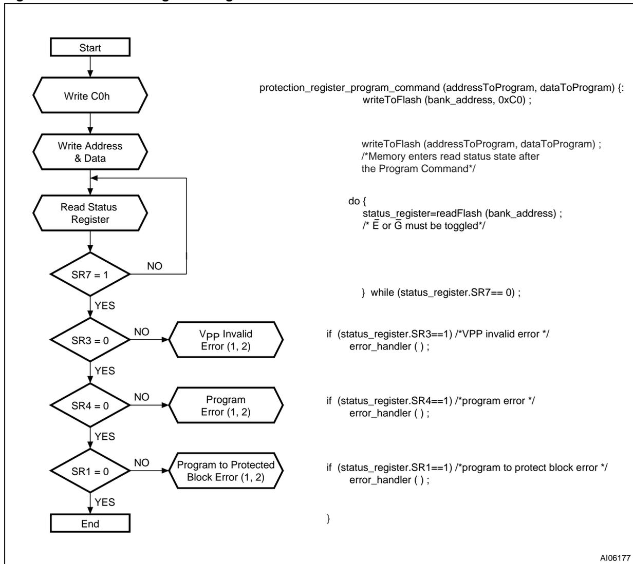
Note: 1. Status check of SR1 (Protected Block), SR3 (V<sub>PP</sub> Invalid) and SR4 (Program Error) can be made after each program operation or after a sequence.
