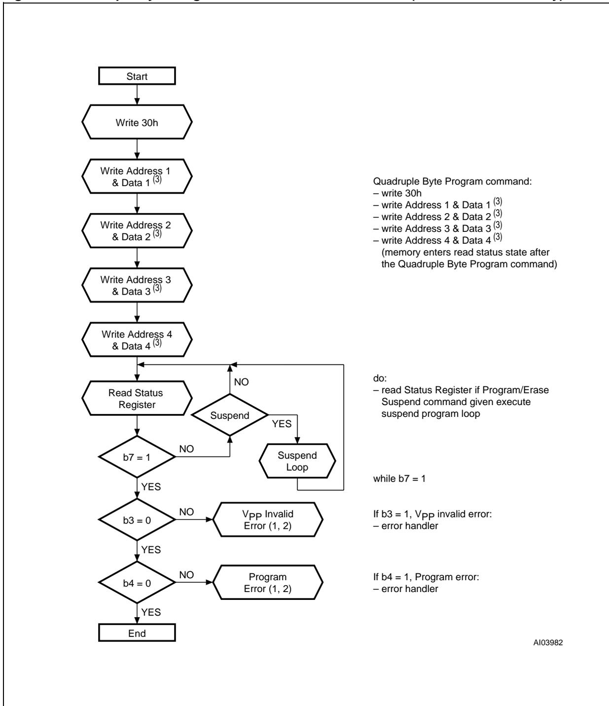
Note: 1. A Status check of b3 (V<sub>PP</sub> invalid) and b4 (Program Error) can be made after each Program operation by following the correct command sequence.
