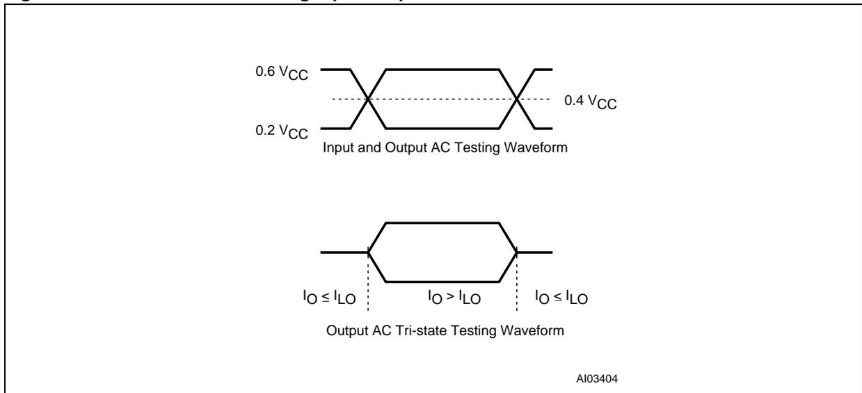
**Table 18. A/A Mux Interface AC Measurement Conditions**
