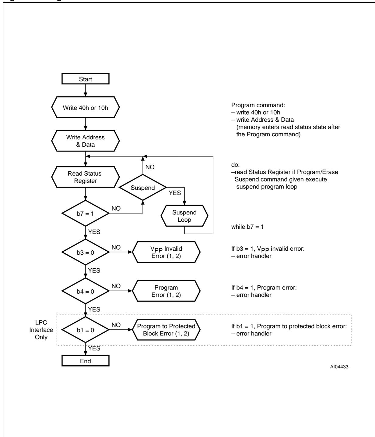
Note: 1. A Status check of b1 (Protected Block), b3 (V<sub>PP</sub> invalid) and b4 (Program Error) can be made after each Program operation by following the correct command sequence.
