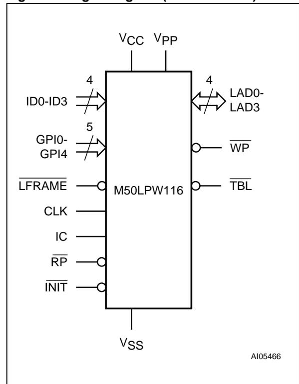
Figure 2. Logic Diagram (A/A Mux Interface)
