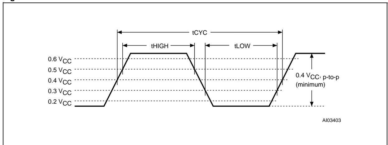
**Table 22. LPC Interface AC Signal Timing Characteristics**
