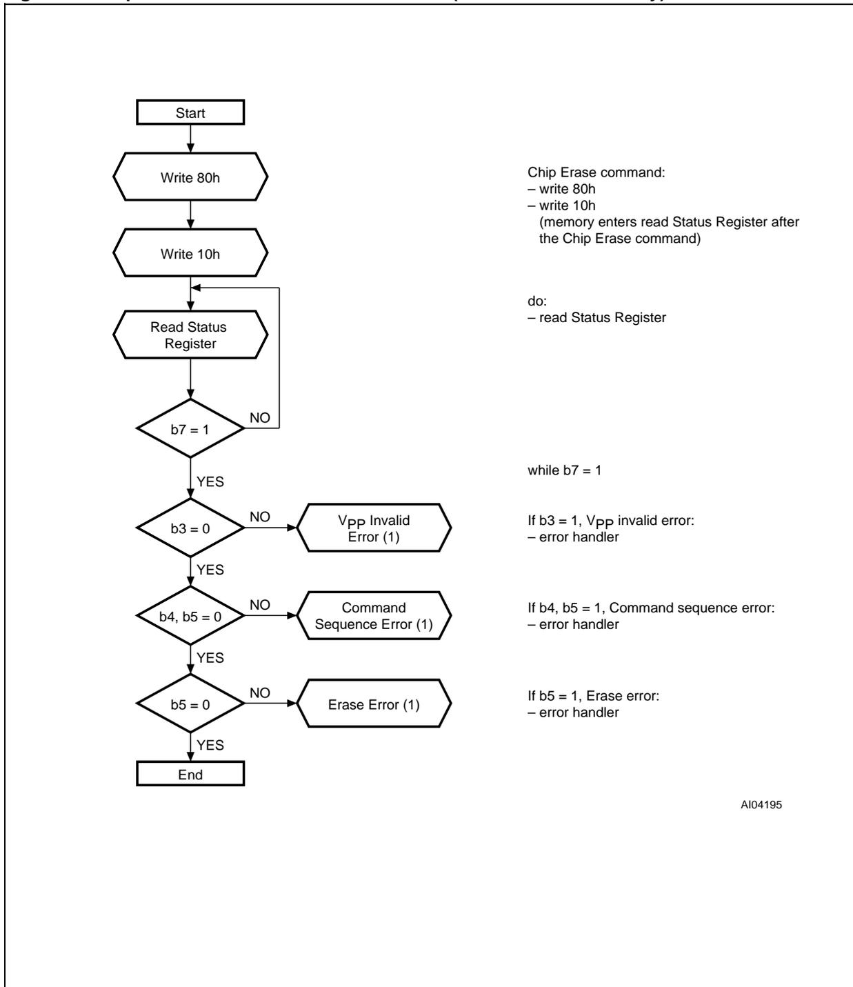
Note: 1. If an error is found, the Status Register must be cleared before further Program/Erase Controller operations.
