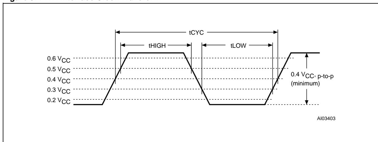
**Table 22. FWH Interface AC Signal Timing Characteristics**
