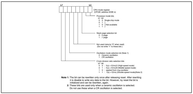
Fig. 8 Structure of CPU mode register
