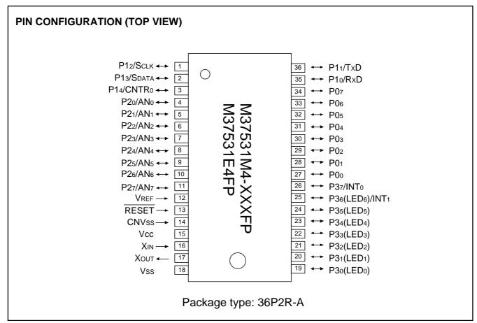
Fig. 1 Pin configuration of M37531M4-XXXFP, M37531E4FP
