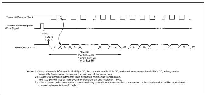
Fig. 24 Continuous transmission operation of UART serial I/O
