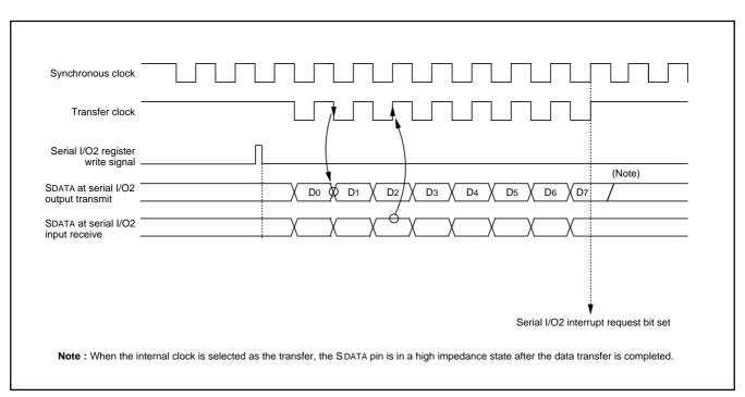
Fig. 28 Serial I/O2 timing (LSB first)
