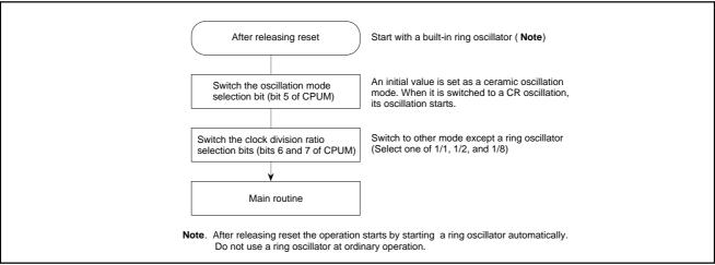
Fig. 9 Switching method of CPU mode register
