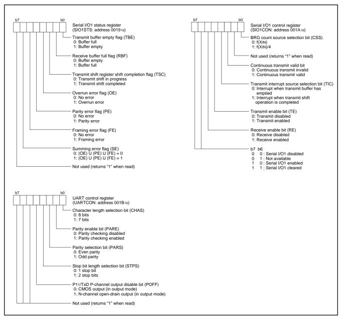
Fig. 25 Structure of serial I/O1-related registers (1)
