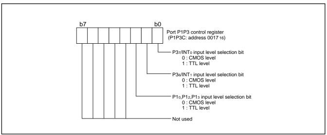
Fig. 13 Structure of port P1P3 control register
