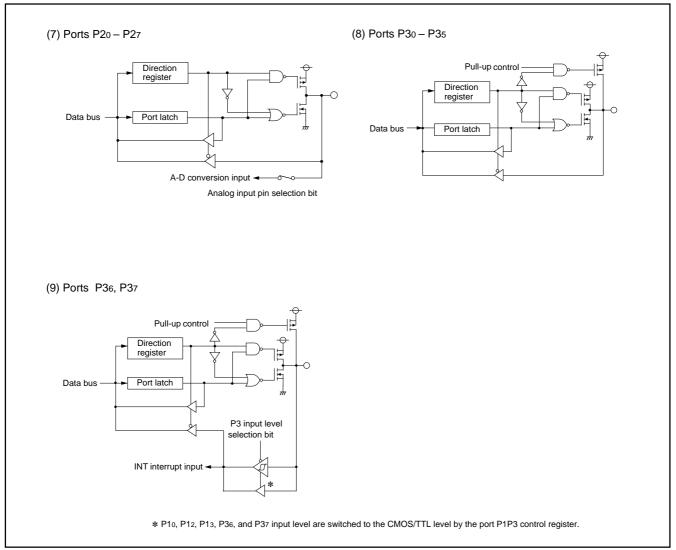
Fig. 15 Block diagram of ports (2)
