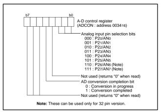
Fig. 29 Structure of A-D control register
