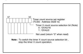
Fig. 20 Timer count source setting register
