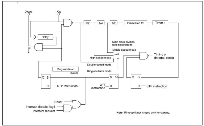
Fig. 42 Block diagram of system clock generating circuit (for CR oscillation)
