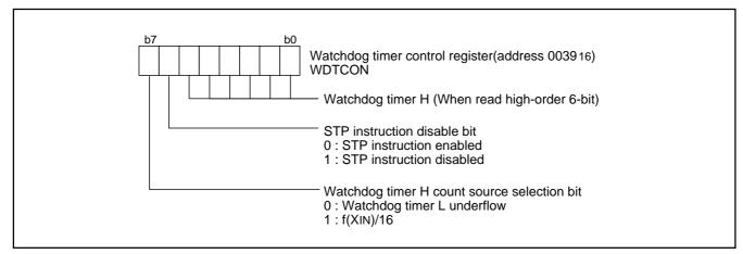
Fig. 33 Structure of watchdog timer control register
