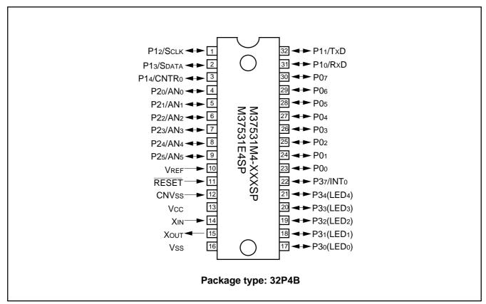
Fig. 3 Pin configuration of M37531M4-XXXSP, M37531E4SP
