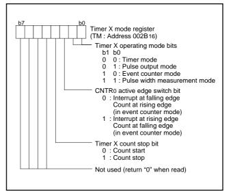
Fig. 19 Structure of timer X mode register
