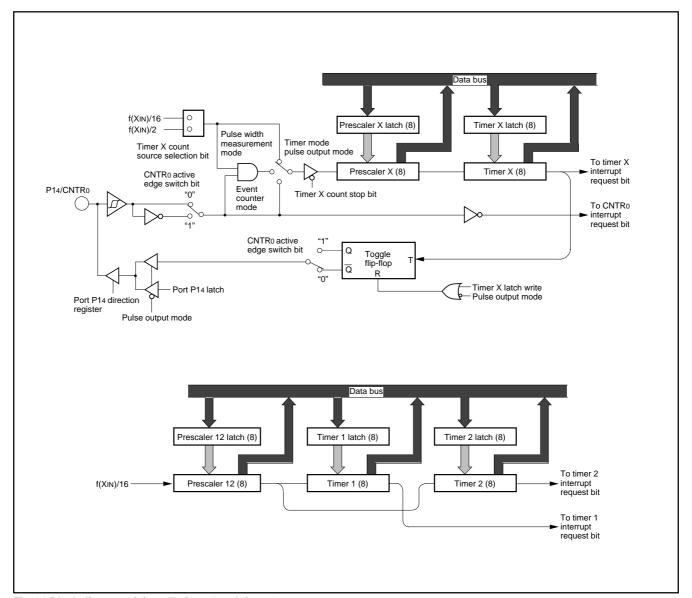
Fig. 21 Block diagram of timer X, timer 1 and timer 2
