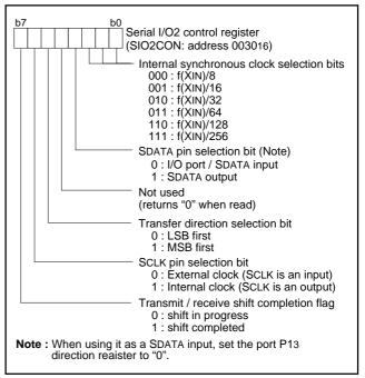
Fig. 26 Structure of serial I/O2 control registers
