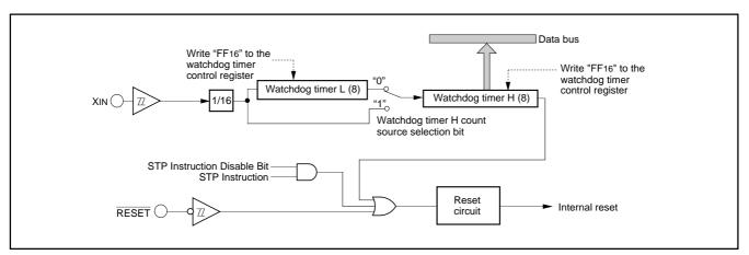
Fig. 32 Block diagram of watchdog timer
