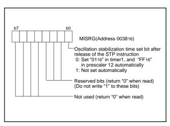
Fig. 40 Structure of MISRG
