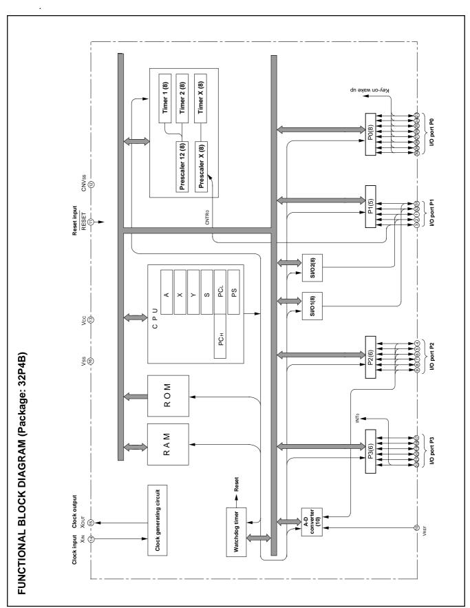
Fig. 6 Functional block diagram (32P4B package)
