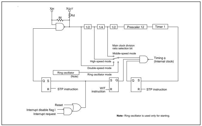
Fig. 41 Block diagram of system clock generating circuit (for ceramic resonator)
