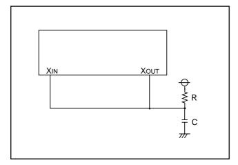
Fig. 38 External circuit of CR oscillation
