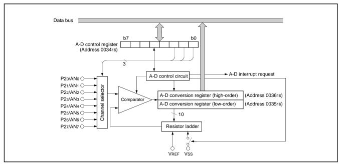
Fig. 31 Block diagram of A-D converter
