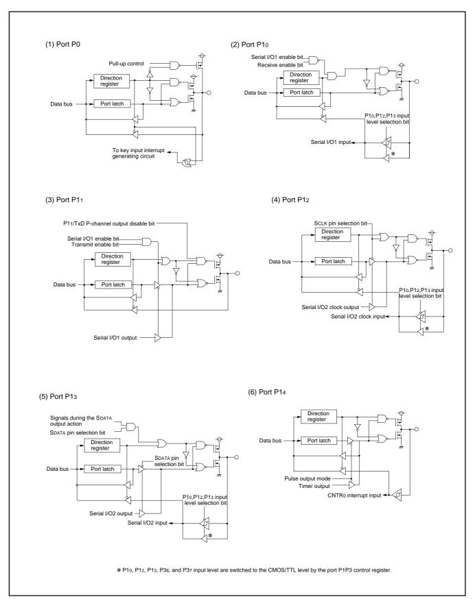
Fig. 14 Block diagram of ports (1)
