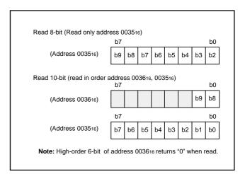
Fig. 30 Structure of A-D conversion register
