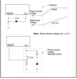
Fig. 34 Example of reset circuit
