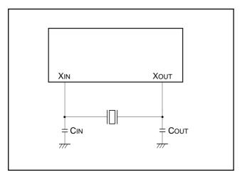
Fig. 37 External circuit of ceramic resonator
