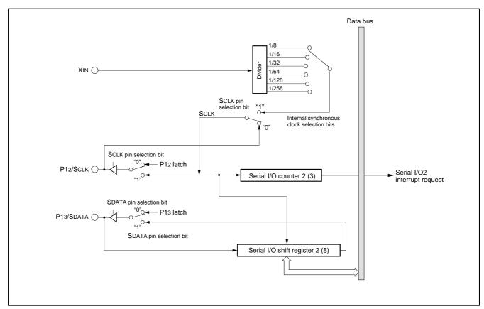
Fig. 27 Block diagram of serial I/O2
