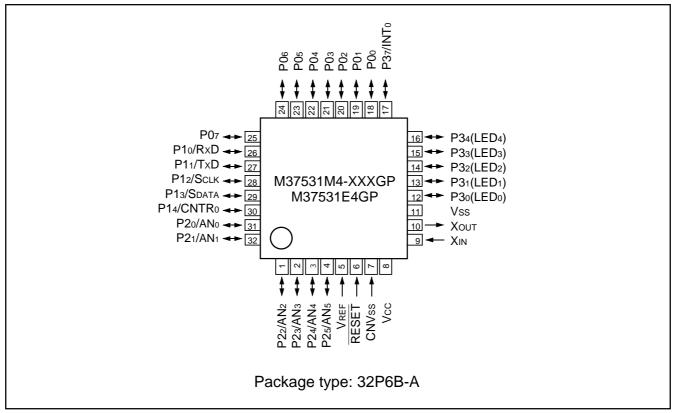
Fig. 2 Pin configuration of M37531M4-XXXGP, M37531E4GP
