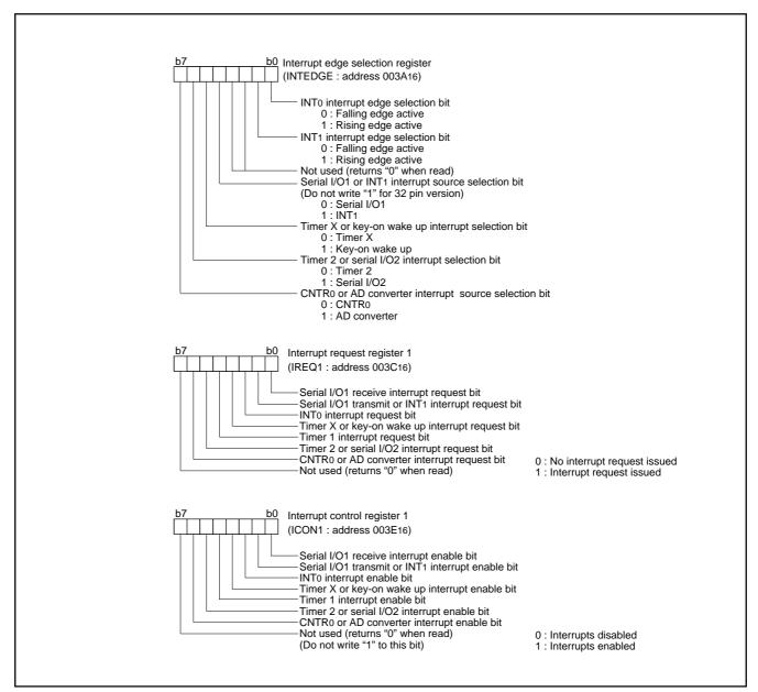
Fig. 17 Structure of Interrupt-related registers
