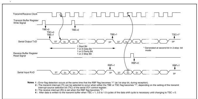
Fig. 23 Operation of UART serial I/O function
