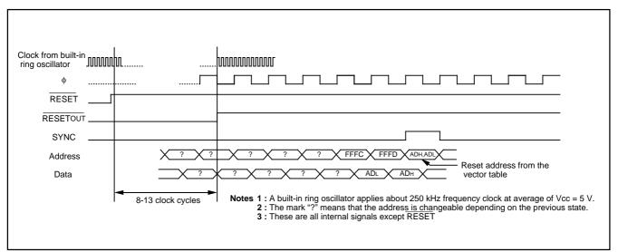
Fig. 35 Timing diagram at reset
