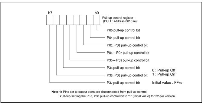
Fig. 12 Structure of pull-up control register
