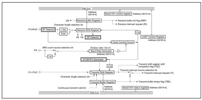
Fig. 22 Block diagram of UART serial I/O
