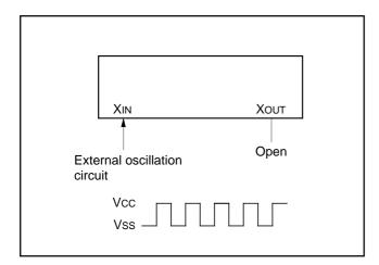
Fig. 39 External clock input circuit
