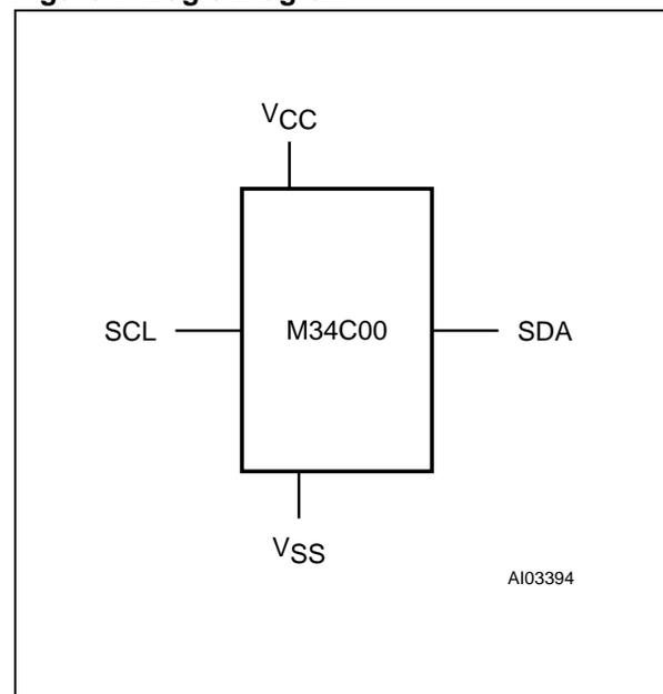
Figure 2A. SO and TSSOP Connections
