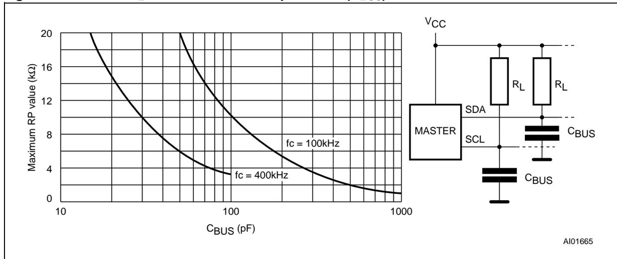
collector signals on the bus. A pull up resistor must be connected from Serial Data (SDA) to  $V_{CC}$ . (Figure 3 indicates how the value of the pull-up resistor can be calculated).
