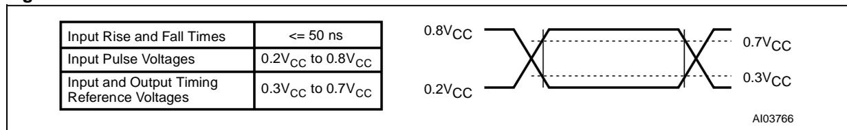
Table 7. Input Parameters <sup>1</sup>( $T_A = 25$  °C,  $f = 400$  kHz)
