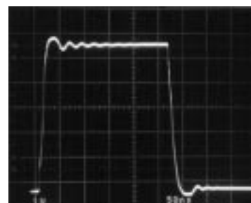
Large-Signal Transient ( A_V = -1 , C_L = 200pF )
