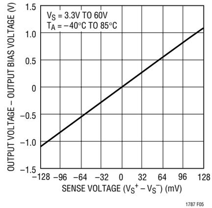
Figure 5. Single Supply Output Voltage with  $V_{BIAS} = 1.25V$
