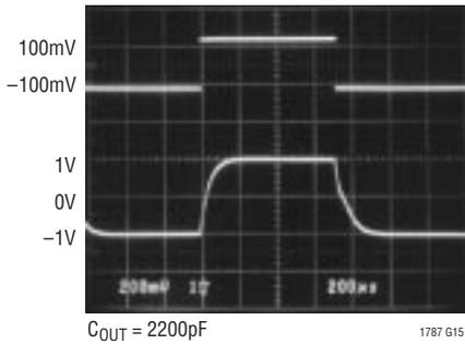
$V_{OUT}$  Error vs Supply Ripple
