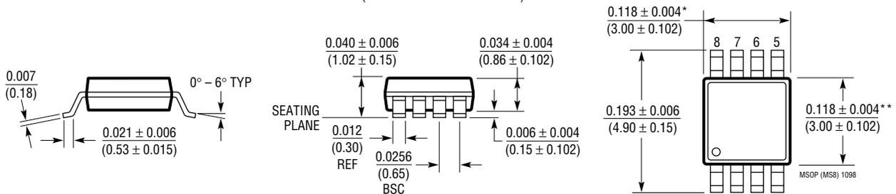
\* DIMENSION DOES NOT INCLUDE MOLD FLASH, PROTRUSIONS OR GATE BURRS. MOLD FLASH, PROTRUSIONS OR GATE BURRS SHALL NOT EXCEED 0.006\* (0.152mm) PER SIDE
