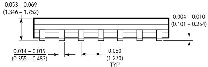
\*DIMENSION DOES NOT INCLUDE MOLD FLASH. MOLD FLASH SHALL NOT EXCEED 0.006\* (0.152mm) PER SIDE
