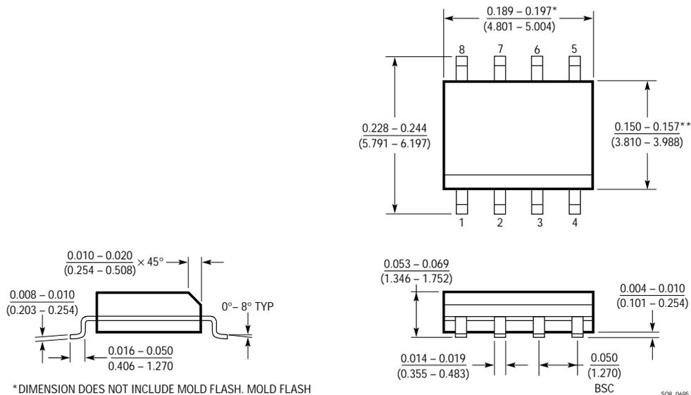
\* DIMENSION DOES NOT INCLUDE MOLD FLASH. MOLD FLASH SHALL NOT EXCEED 0.006\* (0.152mm) PER SIDE
