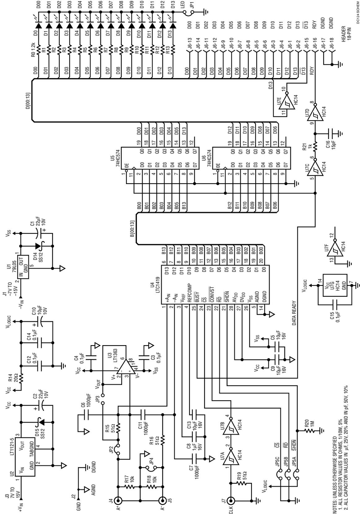
Figure 13a. Suggested Evaluation Circuit Schematic
