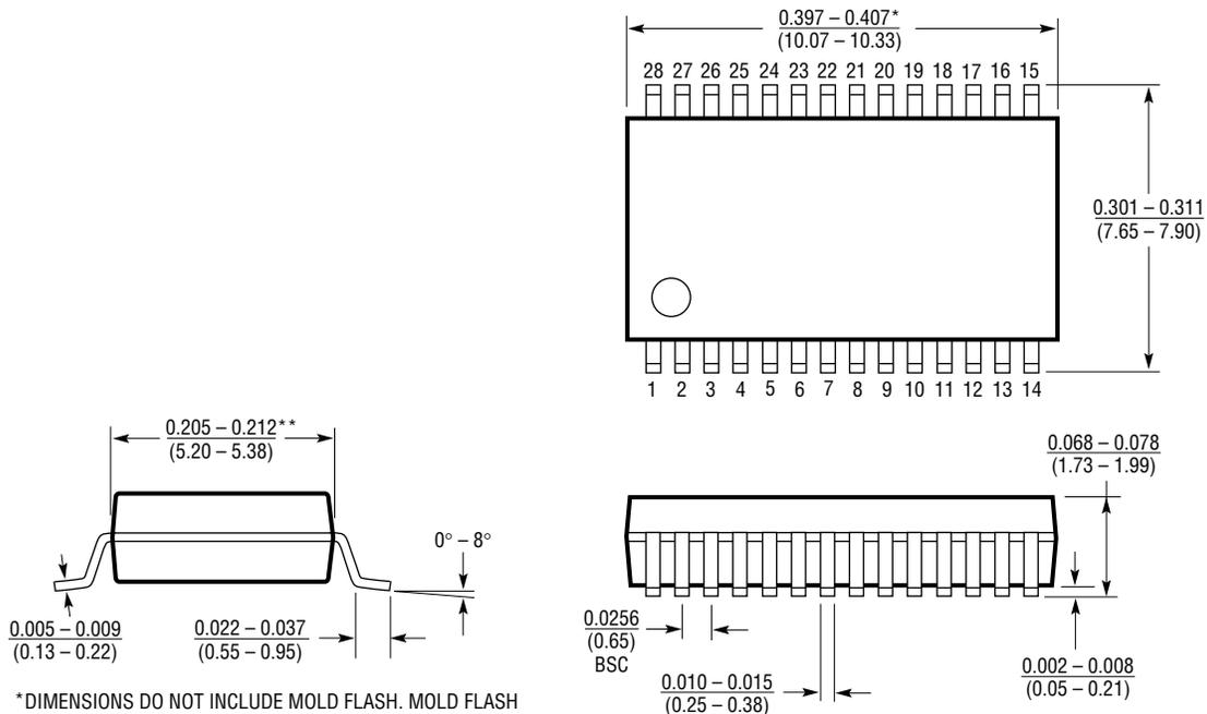
\*DIMENSIONS DO NOT INCLUDE MOLD FLASH. MOLD FLASH SHALL NOT EXCEED 0.006" (0.152mm) PER SIDE
