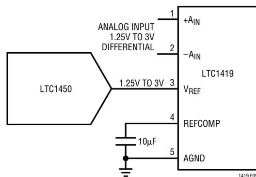
Figure 9. Driving V<sub>REF</sub> with a DAC
