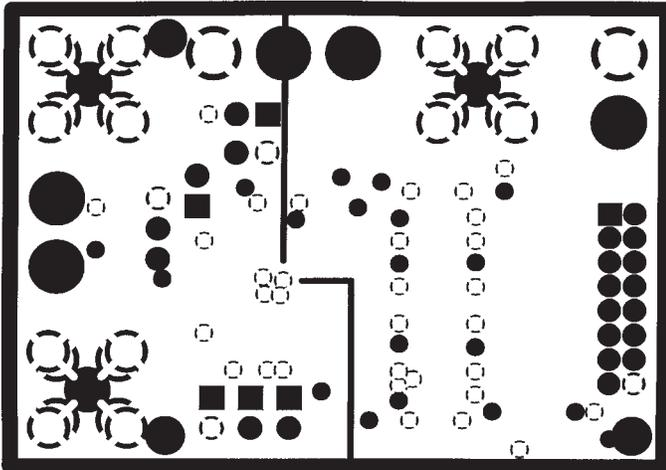
Figure 17. Ground Plane Layer for LTC1405/LTC1420 Demo Board
