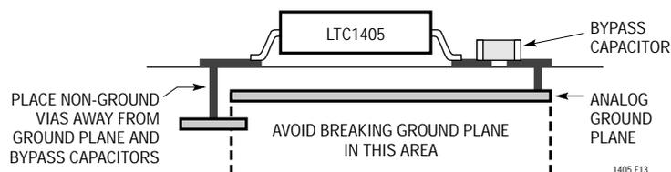
Figure 13. Cross Section of LTC1405 Printed Circuit Board
