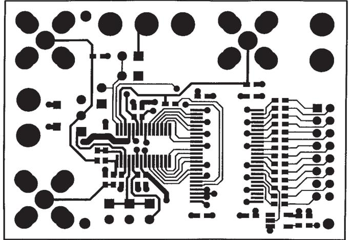
Figure 16. Top Layer for LTC1405/LTC1420 Demo Board
