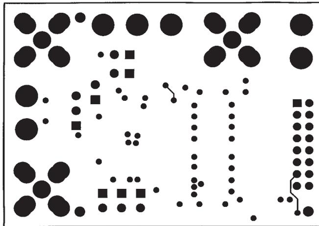
Figure 19. Bottom Layer for LTC1405/LTC1420 Demo Board
