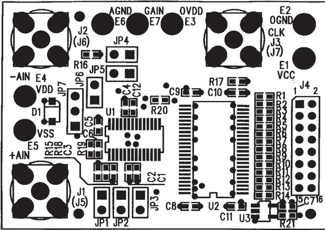
Figure 15. Top Silkscreen Layer for LTC1405/LTC1420 Demo Board
