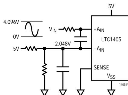
Figure 6. DC Coupling a 0V to 4.096V Signal
