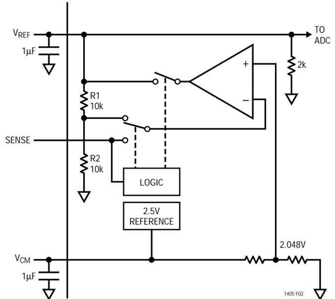
Figure 2. Reference Circuit
