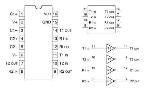
C+ : EXTERNAL CAPACITOR (+TERMINAL)C- : EXTERNAL CAPACITOR (-TERMINAL)
