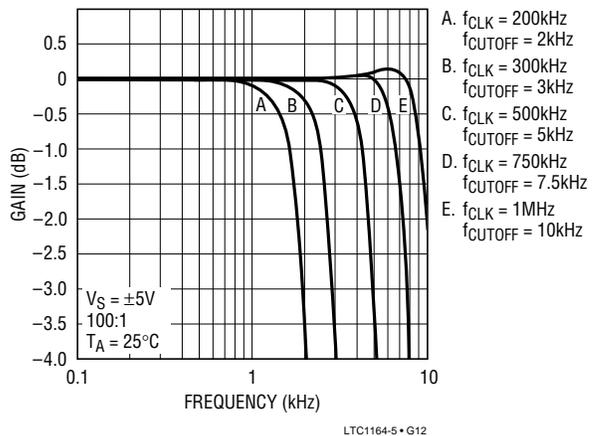
Maximum Passband over Temperature for  $V_S = \pm 5V, 100:1$
